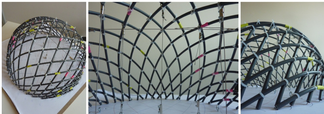
Figure 4.12: Physical modeling of the Flying Dome to analyze the visual effects of the irregular mesh
