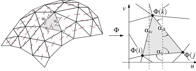
Figure 3: A discrete isothermic parameterization. Angles between triangle edges and a curvature direction family are preserved by the map.
