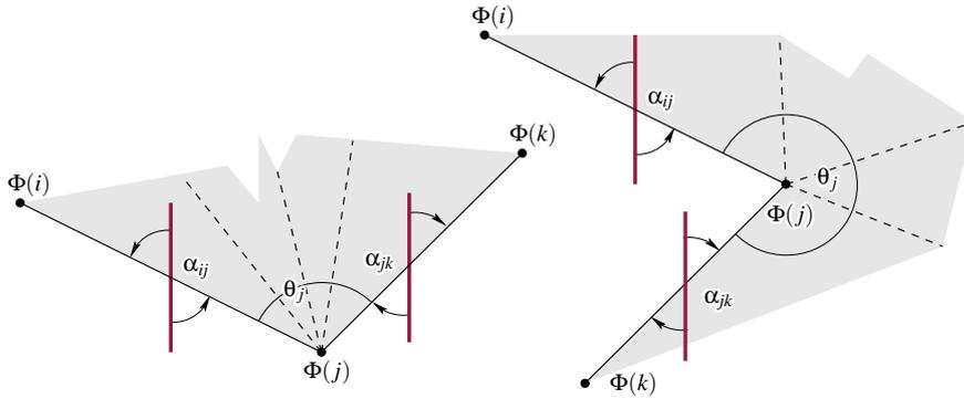
Figure 4: Curvature boundary conditions: In parameter space the interior angle  $\theta_j$  at the vertex  $\Phi(j)$  has to be chosen such that curvature directions given by angles  $\alpha_{ij}$  and  $\alpha_{jk}$  align with the  $v$ -axis. This choice is unique up to addition of  $k\pi$ . The above pictures show two possible layouts in the parameter plane depending on the interior angle sum on the surface.
