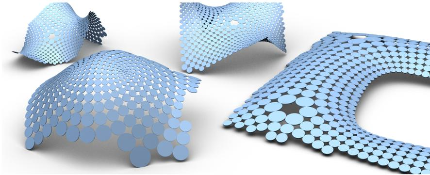
Figure 7: S-isothermic meshes created from the models presented in Figure 2. The inner quadrilaterals are optimized towards touching incircles. A series of touching circles in a row can be interpreted as discrete curvature line.
