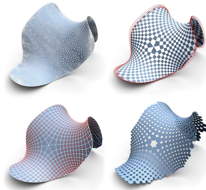
Figure 1: The algorithmic steps of this paper: For a triangulated surface we calculate texture coordinates by solving a boundary value problem for principle curvature directions on boundary edges (checker board texture and red directions). The edges of the corresponding quad mesh align with the curvature directions (red crosses). The mesh is then optimized towards planar quads with touching incircles.
