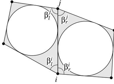
Figure 8: Labels for the touching-circles-functional at an edge. The circles touch if the ratio  $\cot(\beta_l^i/2)/\cot(\beta_r^i/2)$  is equal on both sides of the edge.
